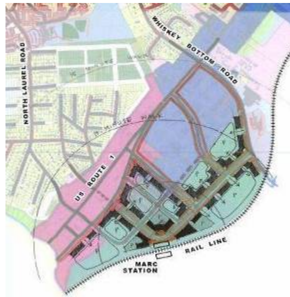
This vision for North Laurel shows new collector roads through the site linking US 1 and Whiskey Bottom road and site design that places buildings fronting the street.
