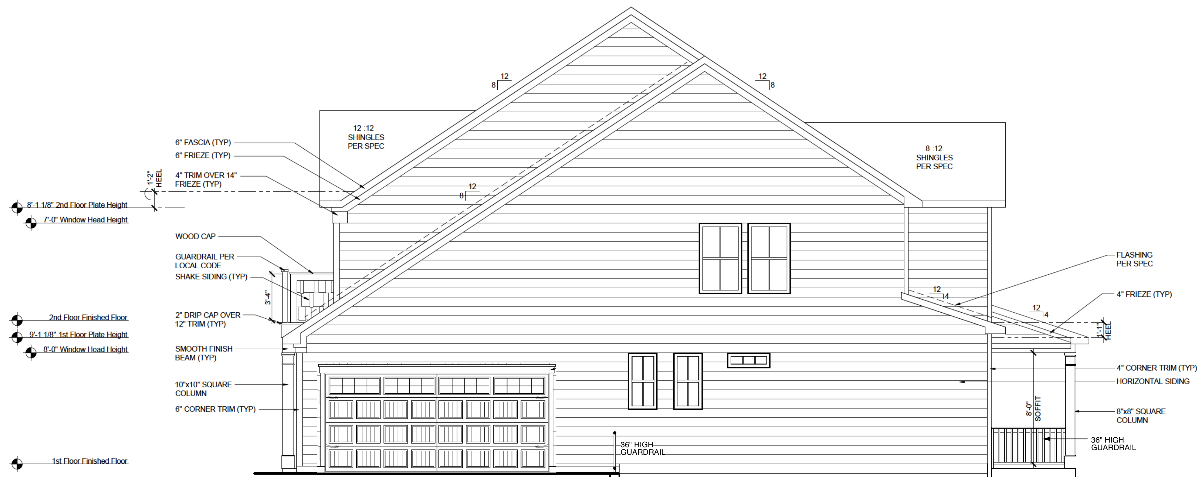
RIGHT ELEVATION - SHL AT END SCALE: 1/8"=1'-0" (11"x17" SHEET SIZE) SCALE: 1/4"=1'-0" (24"x36" SHEET SIZE)
